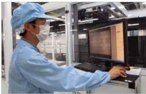
One hundred per cent micro-optical electroluminescent inspection
